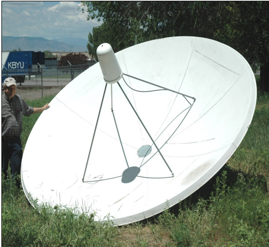
Figure 5-2 Original 4-Meter Antenna donated to Physics and Astronomy Radio Astronomy Research by KBYU Broadcasting. This antenna was later reconditioned, re-purposed, and retrofitted with appropriate HI and OH MASER Imaging LNAs. Additionally a new antenna mount and base was fabricated with tracking hardware installed. Photo, courtesy of Scott Daniel.
