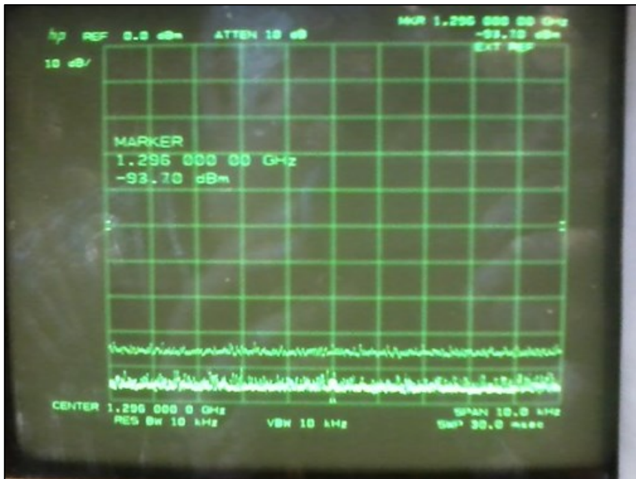
Figure 3-15 Integrated solar transit at 1296MHz over several hours shows -85dBm amplitude peak with instantaneous level of -95dBm.
